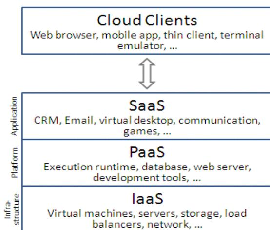
Figure-3 The layers of cloud service models
